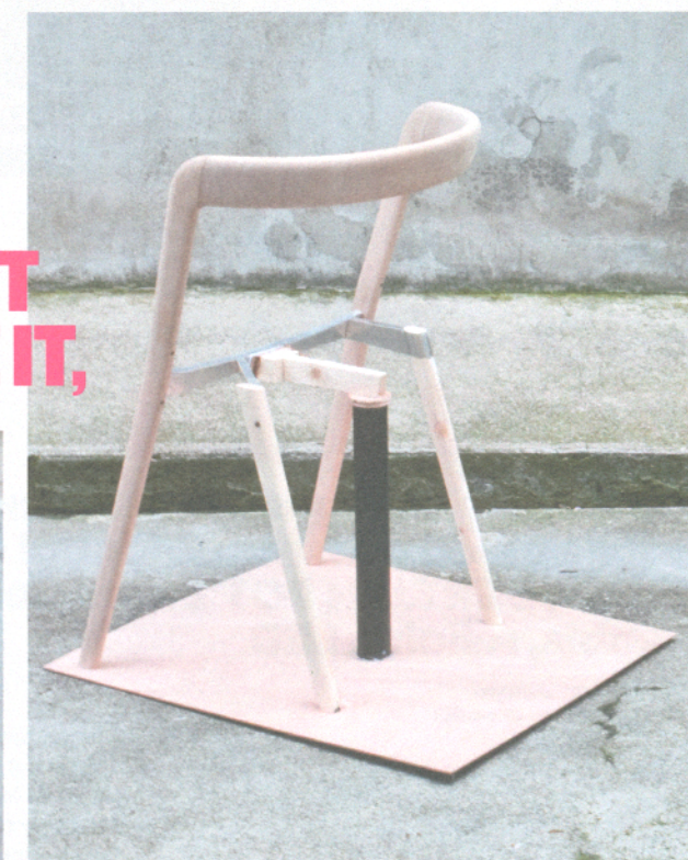
RESEARCH MODELS WERE USED TO REDUCE THE SIZE OF BAGUETTE'S ALUMINIUM FRAME AS FAR AS POSSIBLE.
