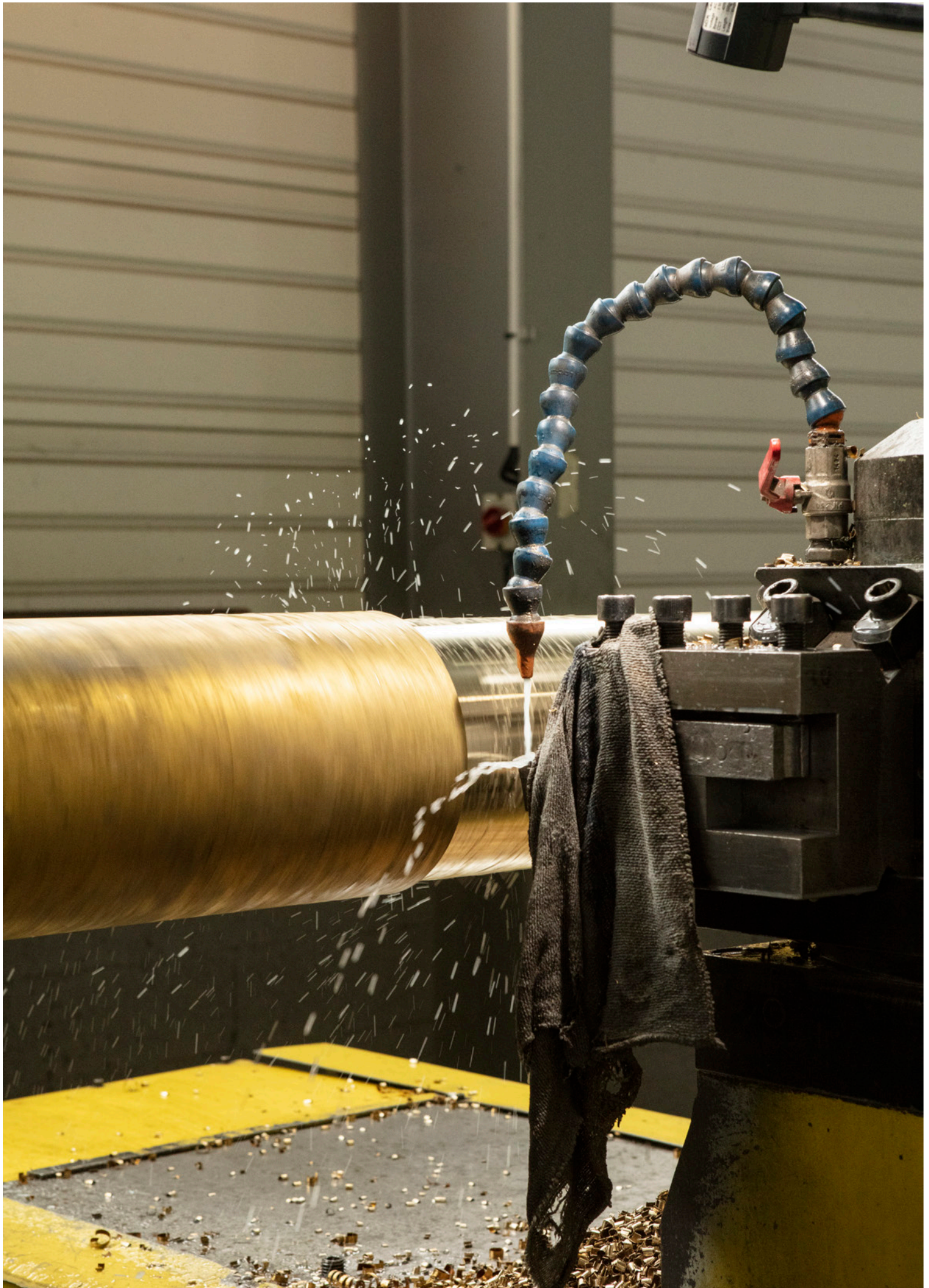
Machining the bronze-aluminium tubes in the LBI workshops in Amneville
