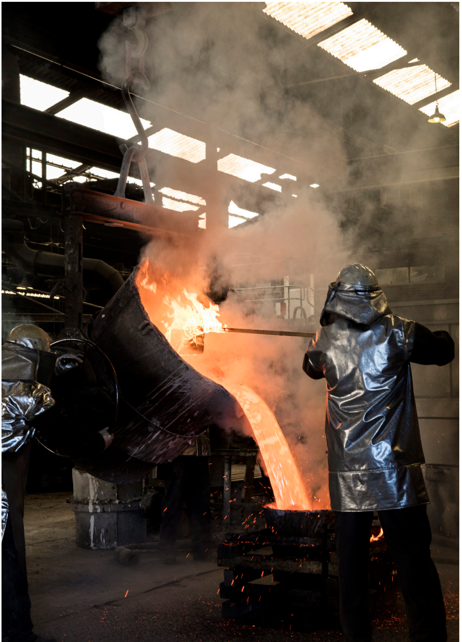
Casting the bronze-aluminium tubes
