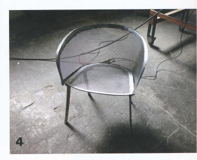
An injection-moulded ring connects Stampa's seat to its back and armrests, and hydroformed legs support the shell.
