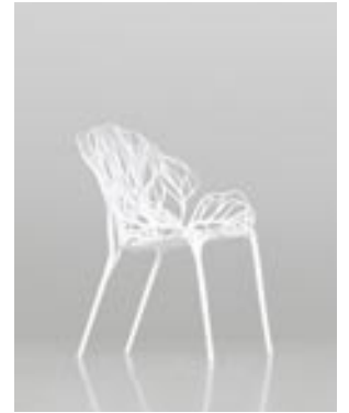
5 Stereolithographic model, scale 1:5, November 2005. The first three-dimensional model made from a three-dimensional data file.
